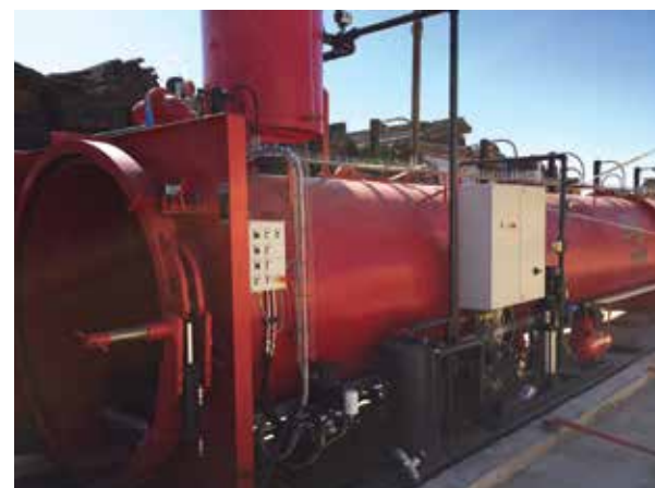
▲ Photo 14 : Autoclave © P. Filius, ARCH TIMBER PROTECTION LTD
